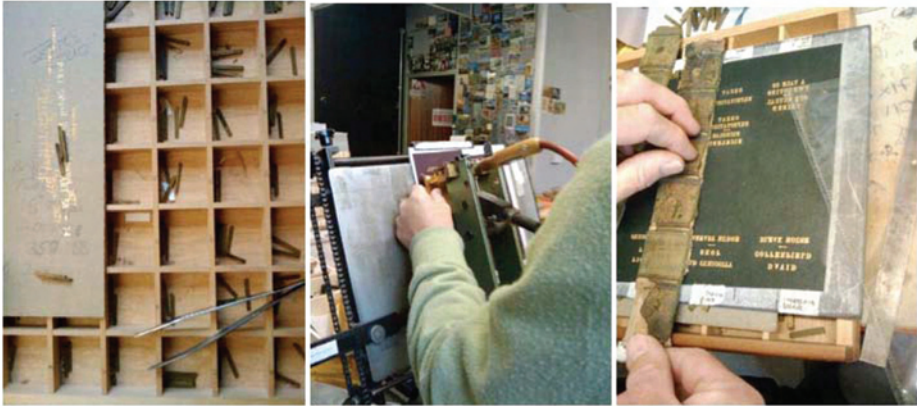
Figure 5. (a) metal type in type trace; (b) type holder and blocking machine; (c) comparing the label of the original spine with the newly printed spine label. This system requires the manual arrangement of cast metal 'blocks' from a typeface family in a 'type holder'. The holder is then secured to the blocking machine, aligned with the cloth, prepared with metal foil, and pressed into the cloth or leather. © Photographs Daniela K Rosner and Alex S Taylor.
