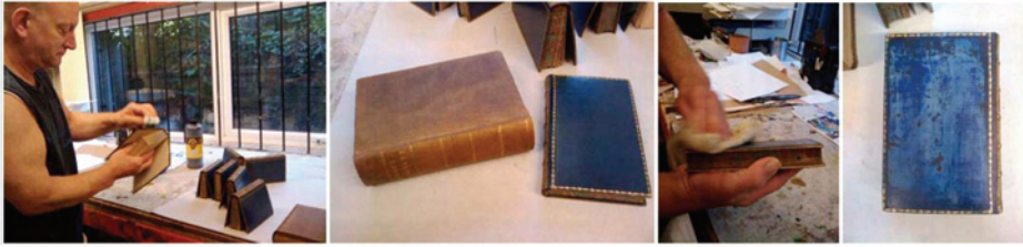
Figure 7. (a) Peter rubs stain on a book cover; (b) old and newly stained books; (c) Peter rubs methylated spirits to remove stains; (d) newly ‘aged’ book. © Photographs Daniela K Rosner and Alex S Taylor.
