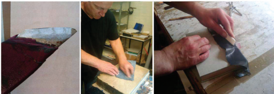
Figure 4. (a) paring knife; (b) Peter pares leather for a book spine; and (c) attaches it to cover boards. © Photographs Daniela K Rosner and Alex S Taylor.
