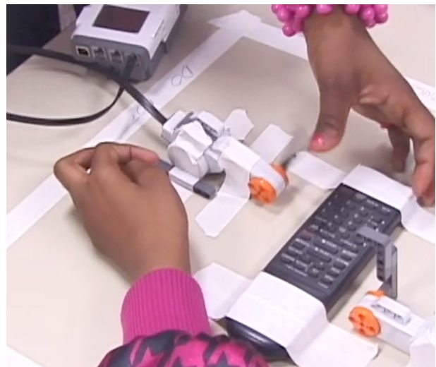
Figure 5. Group 1 focused on the remote control, using one P.Pod to press “On,” another to press “Play”. They mounted the devices with masking tape.
