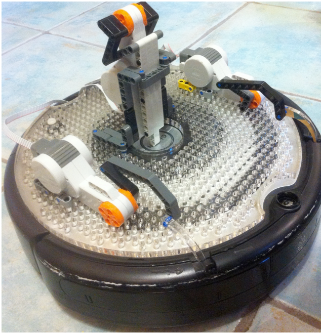
Figure 4. Three robotic P.Pods together mechanically hijack an i-Robot Roomba. A P.Pod poker uses the on/off button to start or stop the motion of the Roomba. Side-mounted P.Pods pinch the bumpers, giving the Roomba false collision input, causing it to turn away from the side of the pinched bumper.
