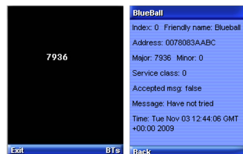
Figure 1. BTScores; the main window and a window holding more details on a specific device, here an Arduino board named the BlueBall
