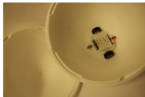
Figure 4. The BlueBall flipped open revealing the Arduino Bluetooth master device.
