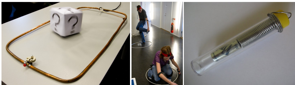
Figure 2. The diZe – a playful presentation of the reading angle of RFID; BendID – a bit where the user wears tags over her whole body; A mechanical model of an accelerometer showing how gravity always is a factor
