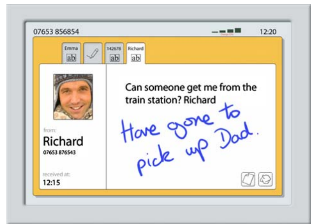
Fig. 5 The HomeNote interface showing a text message overlaid with a scribbled note
